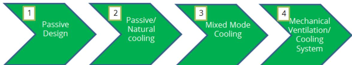
Figure 5: The Cooling Hierarchy- adapted from Cambridge Sustainable Design and Construction SPD, 2020
