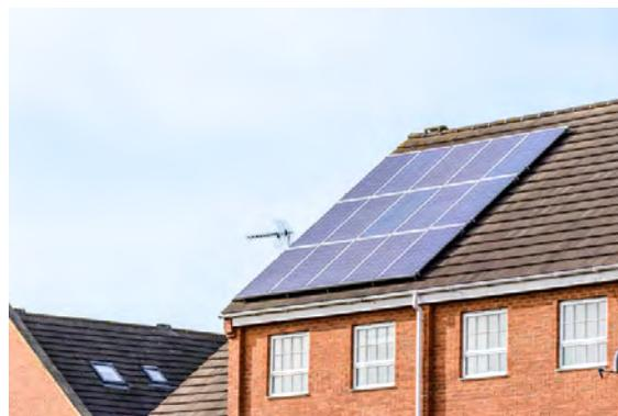
Photovoltaic panels generating electricity. Alternatively solar thermal roof panels can be used to generate hot water.
